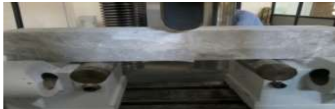
Fig.4.7 Flexure test of specimen
