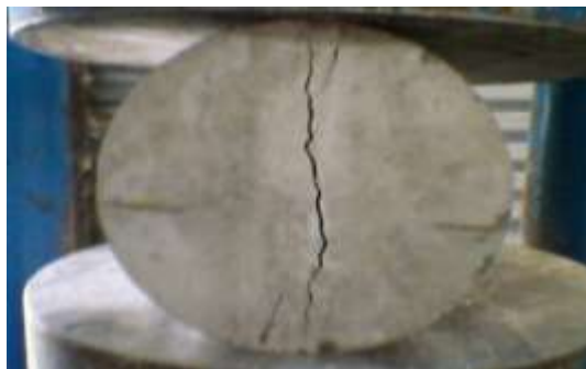
Fig.4.4 Split tensile test of specimen
