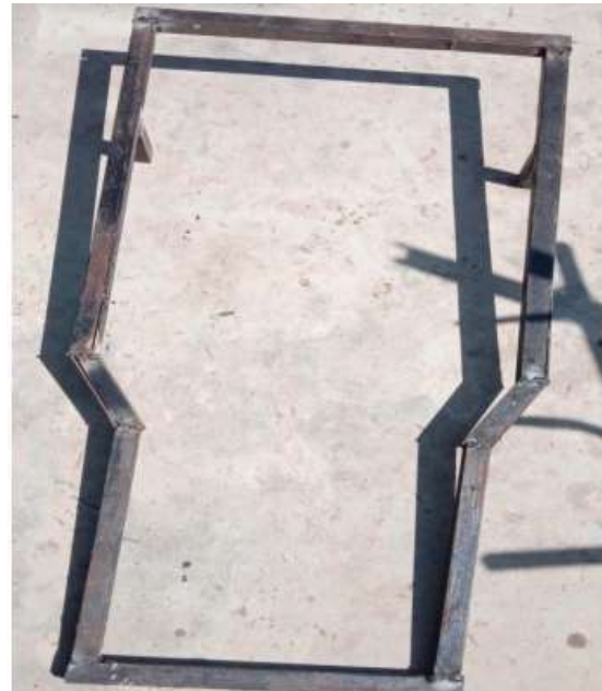
Figure.6 Chassis of the Vehicle Fabrication of the Ploughing Tool and Frame
