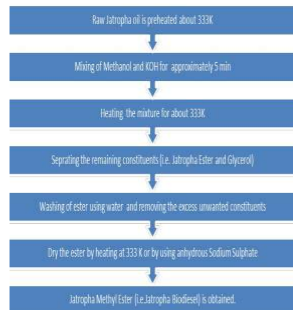
Fig. 2:- Flowchart showing steps in production of Jatropha Biodiesel
