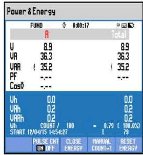
Fig. 4 Power and Energy Measurement Using Fluke
