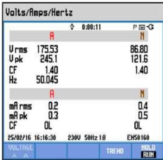
Fig. 3 Voltage and Current Measurement Using Fluke
