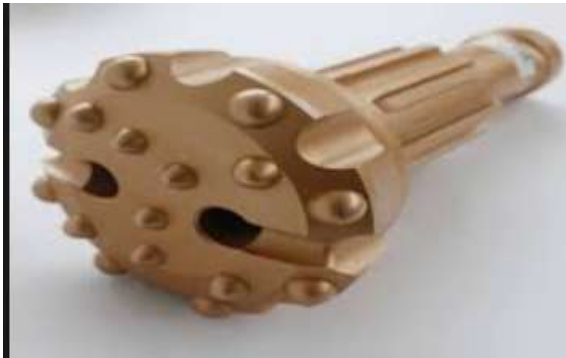
Figure: Down the hole (DTH) Drilling Down the hole hammer:
