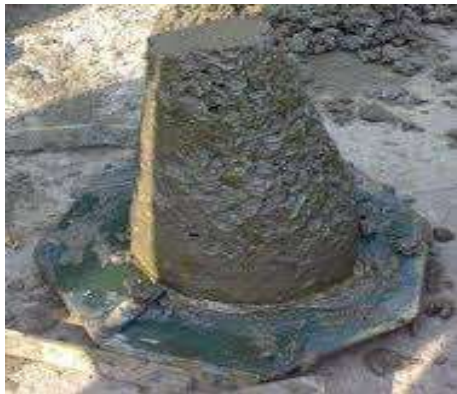
Slump Cone Test
