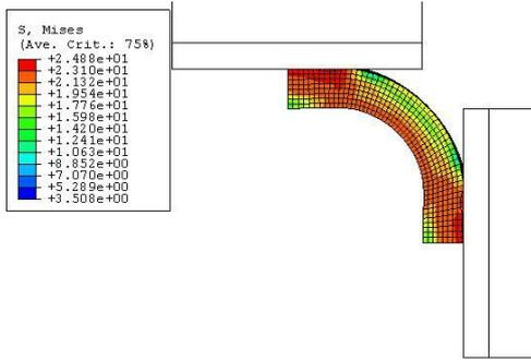
Figure 2. Tube deformed shape after passing through rolls.
