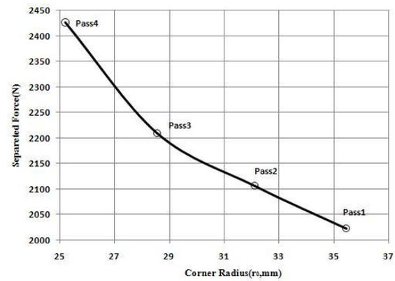
Figure 6. Separated force versus tube corner radius.
