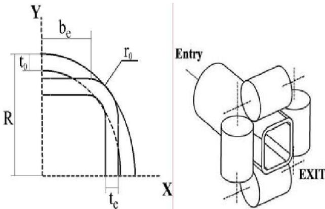
Figure 1. Shape rolling process deformation zone.
