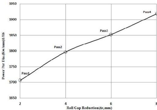
Figure 4. Power dissipated versus roll gap reduction.
