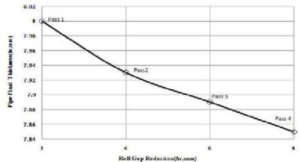
Figure 7. Final rolled tube thickness versus roll gap reduction.
