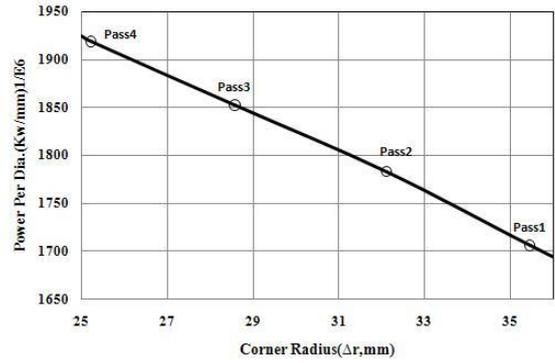
Figure 5. Power dissipated versus tube corner radius.
