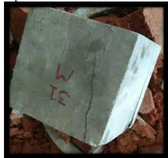
Cubes immersed in HCL for 90 Days IMMERSION OF CIJBES CASTE WITH FIBERS AND WITHOUT FIHERS IN H 2 SO 4 :
