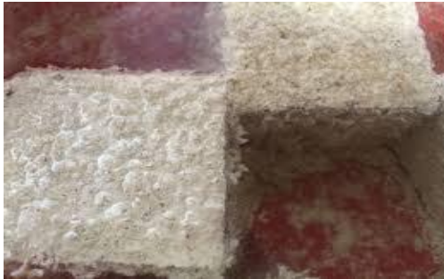
Cubes immersed in H 2 SO 4 for 28 Days
