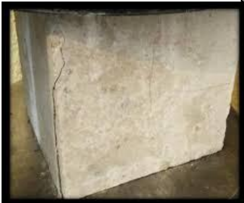
Cubes immersed in HCL for 28 days
