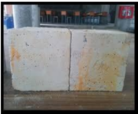
Cubes immersed in HCL for 28 days
