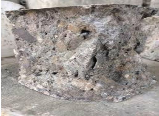
Cubes immersed in H 2 SO 4 for 28 Days
