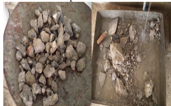
Crushing and washing of demolished concrete Sieve analysis on recycled aggregates-12.5 mm down size
