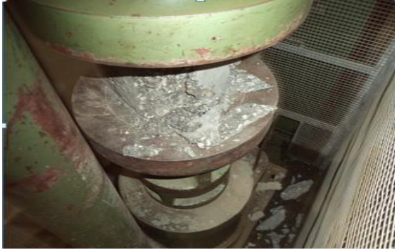
Compression test on cubes
