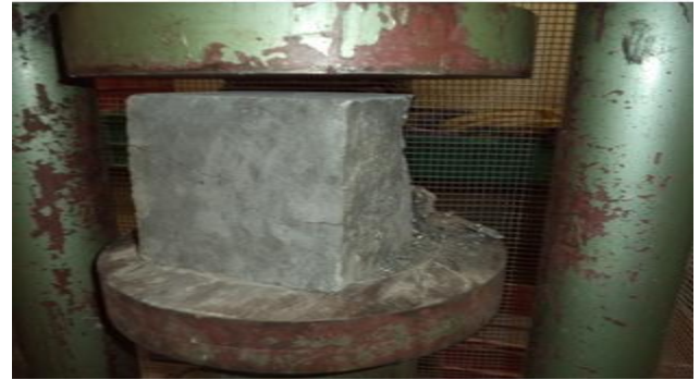
Crushed specimen after test
