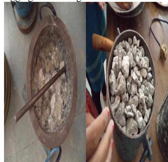
Recycled aggregates subjected to crushing test
