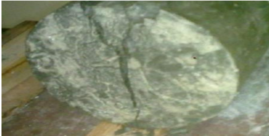
Split tensile strength results of concrete
