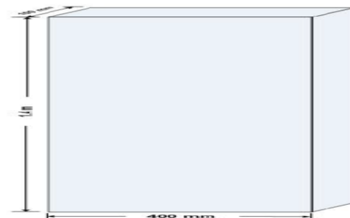
Dimensions of wall element (1400 mm x 400 mm x 100 mm)
