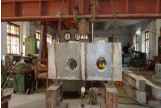
Figure: U-wrap FRP wrapped at Beam 2
