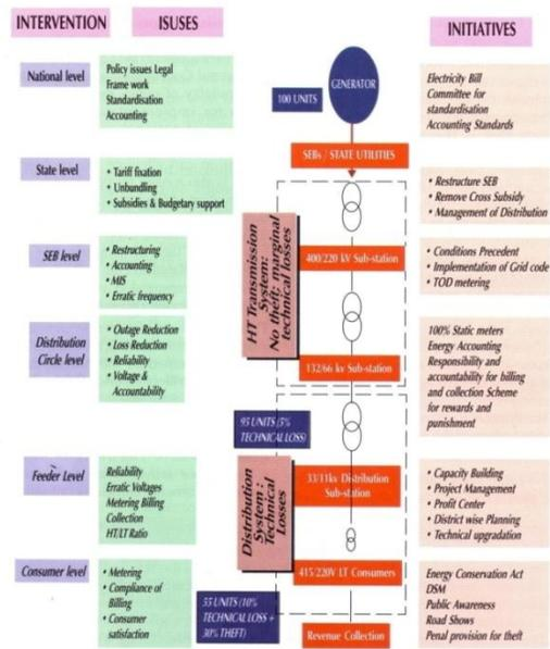
Fig 6:33 KV Distribution System To Lt Consumer
