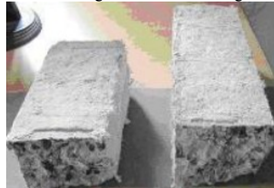
View of Failed Beam
