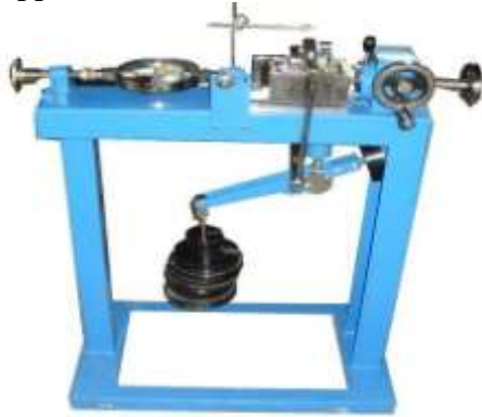
Fig: 3.4 Direct Shear Test Apparatus 3.5.3 California Bearing Ratio (CBR)
