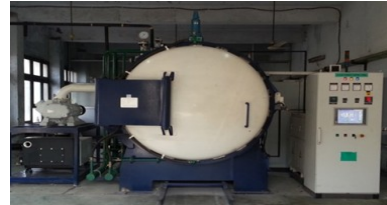
Fig: 3 - Vacuum Hardening Furnace
