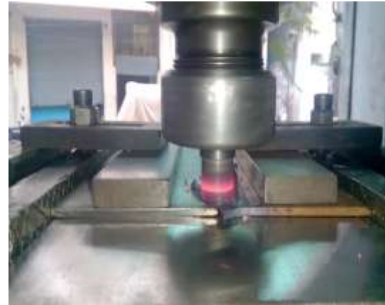
Fig.4.4 Joining of SS316L and Pure copper along the middle line
