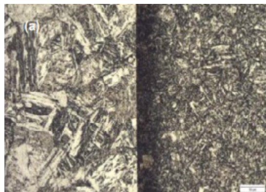
Welded interface joint
