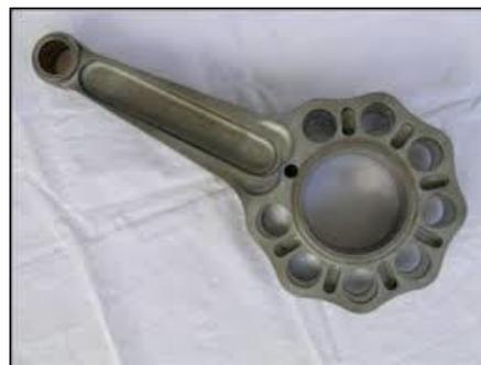
**Fig 1.** Schematic model of master connecting rod.
