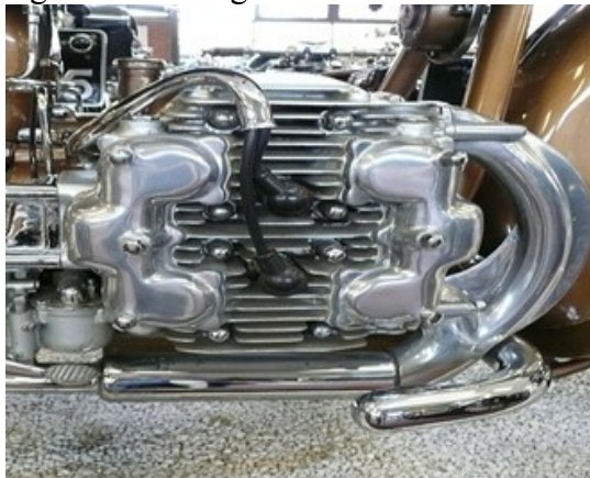
Figure 3.2 longitudinal straight of h-shape engine at the rear of a Fiat 500
