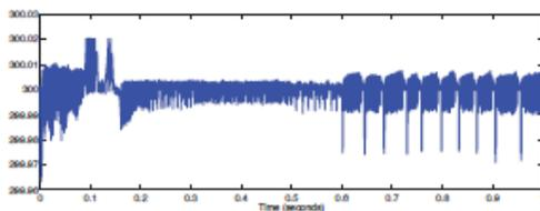
Fig. 13: DC link voltage (V)
