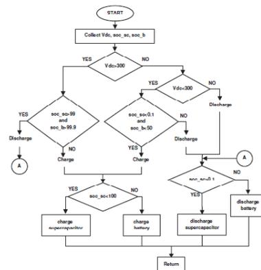
Fig. 2: Flowchart of Charge-Discharge Algorithm
