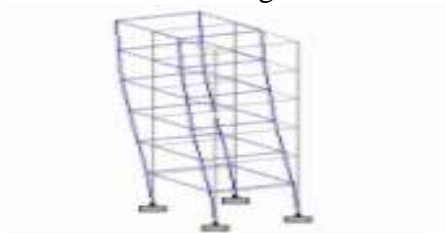
The Fig 4.2 Shows That Torisinal Mode Of Y-Direction In Rc Building
