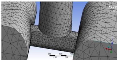
**Fig.2.1: Meshed model Fig. 2.2 Zoomed Meshed Model at the Gates**
