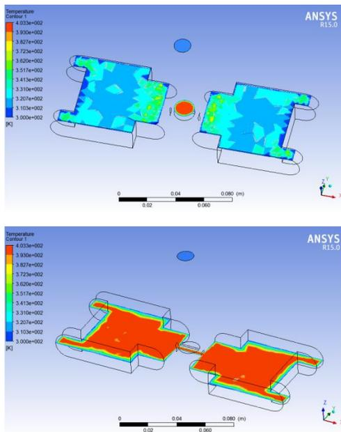
**Fig 3.3 At the Top section, Temperature Contours in horizontal plane at mold.**
