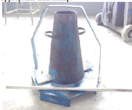
Figure shows Apparatus to determine the workability of concrete (slump test)
