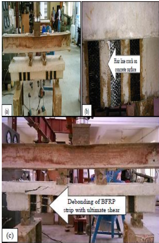
Figure 4.4 (a) Experimental Setup of beam SB4 under four-point loading system, (b) Hair line crack started in shear region at a load of 65kN, (c) Ultimate failure of beam SB4 by debonding of BFRP strip followed by diagonal shear crack
