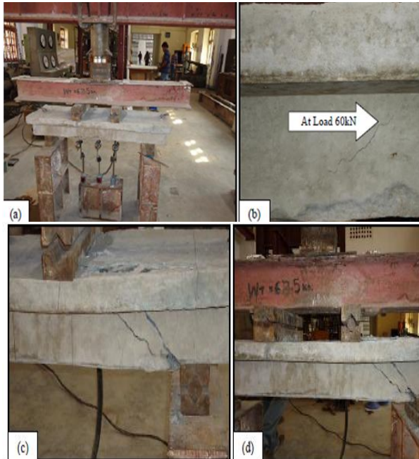
Figure 4.1 (a) Experimental Setup of CB under four-point loading system, (b) Hair line crack started in shear region at a load of 60kN, (c) Crack pattern near Right support, (d) Crack pattern at ultimate failure
