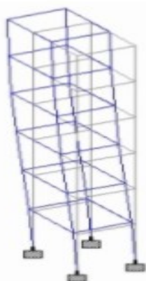
The Fig 4.3 Shows That Torisinal Mode Of Y-Direction In Rc Building
