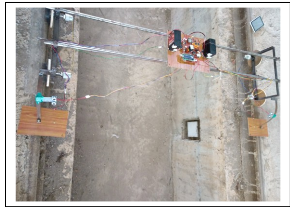
Figure 2. Technical railway crack detection system (Advanced Niyantaran)
