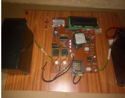
Figure 3. The heart of railway crack detection system (Advanced Niyantran)
