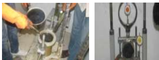
Preparation of mixture and packing the mould & Stability and flow test
