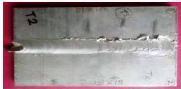
Fig 6: Singlepass with triangle tool
