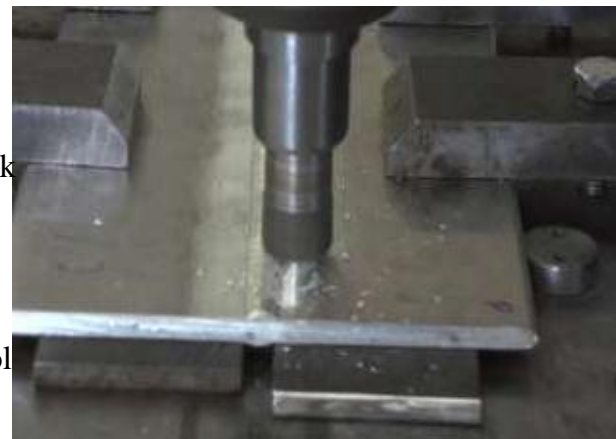
Fig 4: Friction stir welding process
