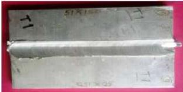
Fig 5: Singlepass with conical tool
