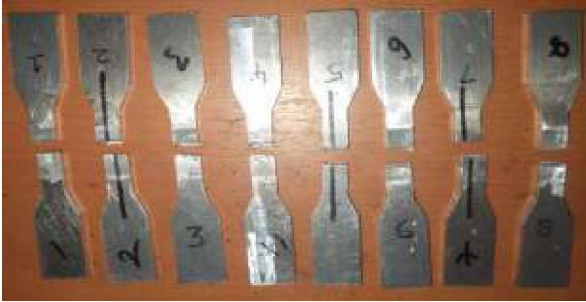
Fig 16: Fractured specimens after tensile test
