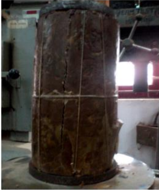
Testing of durability sample after 14 days dry curing
