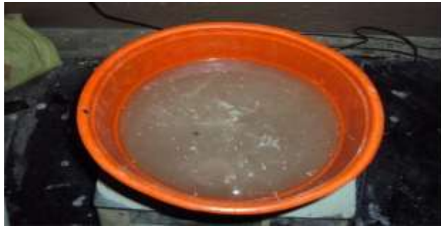
Figure 1: Mixing of sodium silicate and sodium hydroxide solution
