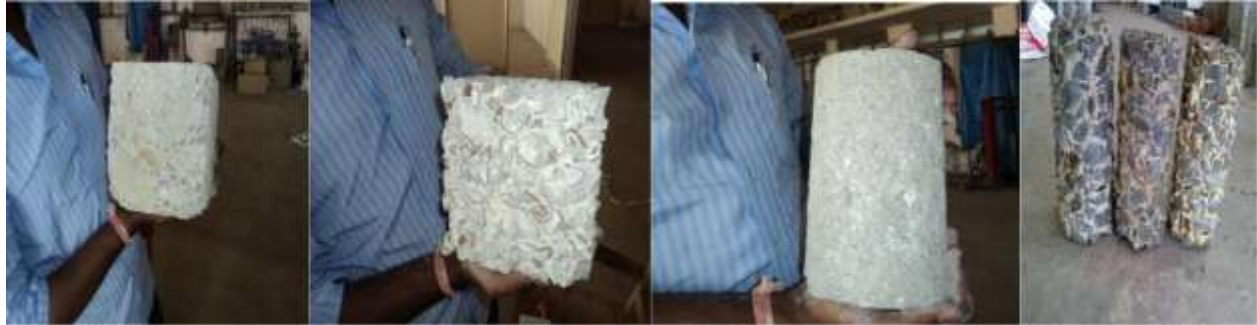
Figure 4: GPC and PPCC specimens exposed to Sulphuric acid solution after 45 days
