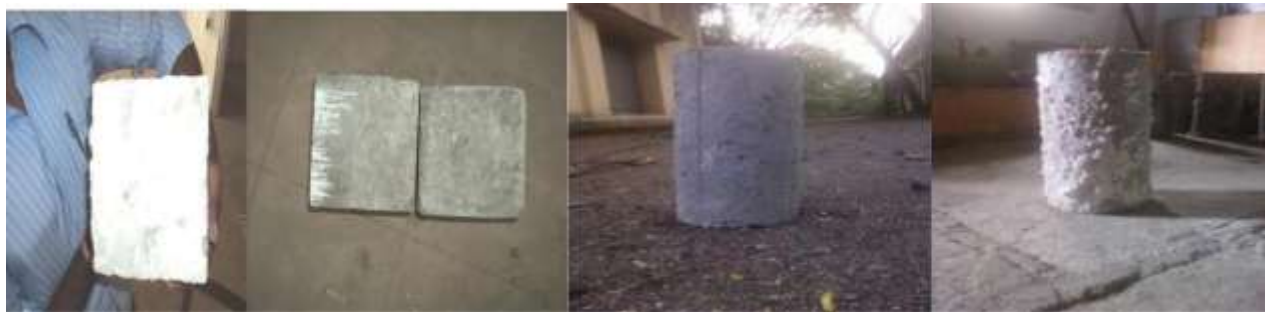
Figure 5: GPC and PPCC specimens exposed to magnesium sulphate solution after 45 days
