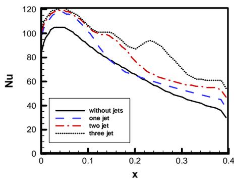
Fig. 4 Local Nuselt number variation on the lower hot wall for different values of expansion ratio,  $Re_m=40000$  and  $Re_j=14000$
