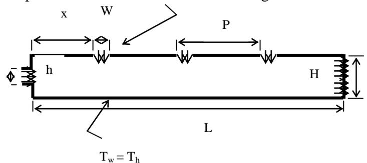
Fig1.schematic diagram of the problem, H=0.05m, L=0.4m, x=0.0492m, H/W=11 and P/W=4
