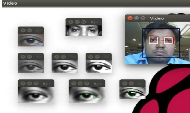
Fig. 8. The center of Eye pupil and circle detection output
