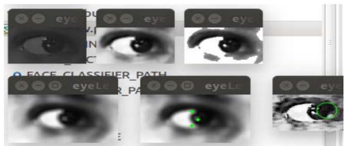
Fig. 7.3. Locate the Eye pupil in right direction
