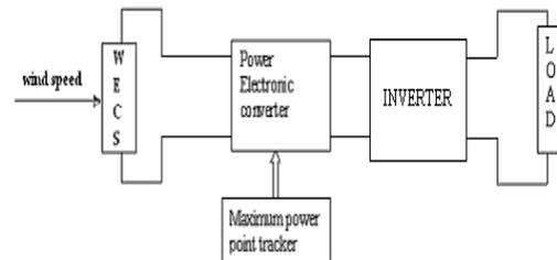
**Figure 2:** Block Diagram for Maximum Power Point Tracking
