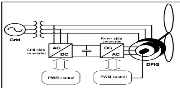
**Figure 1:** Conversion System of Wind Energy
