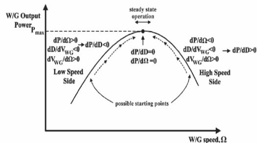
Figure 4.MPP tracking process.
