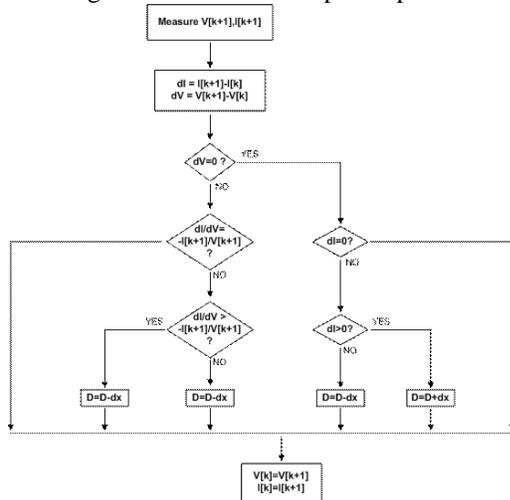
**Figure 6. The Method of Incremental Conductance**
