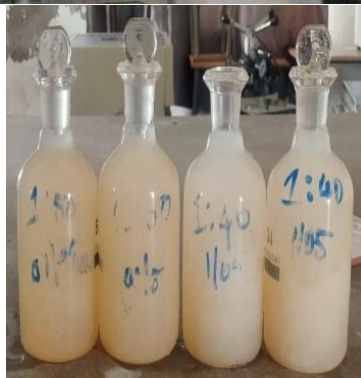
Figure 6: Incubation of samples for BOD/DO
