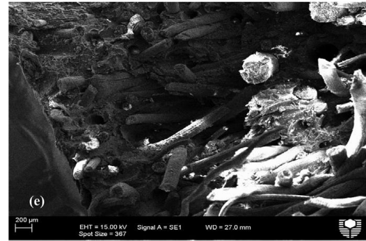
Fig 10: SEM micrographs of PLA based biocomposites reinforced with 20 wt% untreated coir fibres [Yu Dong et.al. 2014].
