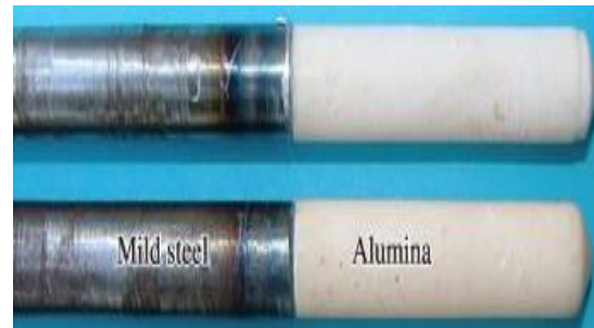
Figure 3.2: Alumina and steel weld joints
