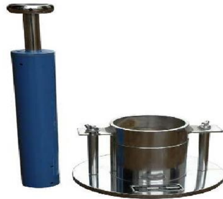
Fig 3.1. Modified Proctor test apparatus
