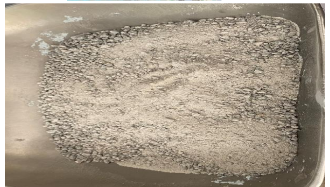
Fig. 2.3.4 Pycnometer with wet Stone Dust and Stone Dust in a tray
