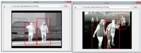
Figure 12. Processed frame of IR Night vision Camera and People are detected and labelled by Red rectangle
