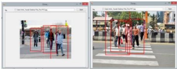
Figure 13. Processed frame of day time normal Camera and People are detected and labelled by Red rectangle
