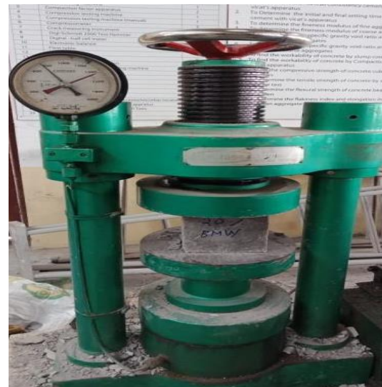
Fig. 6: Compressive strength testing of cube sample.
