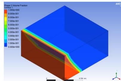
**Fig.4.5** Volume fraction of liquid at 1.3sec
