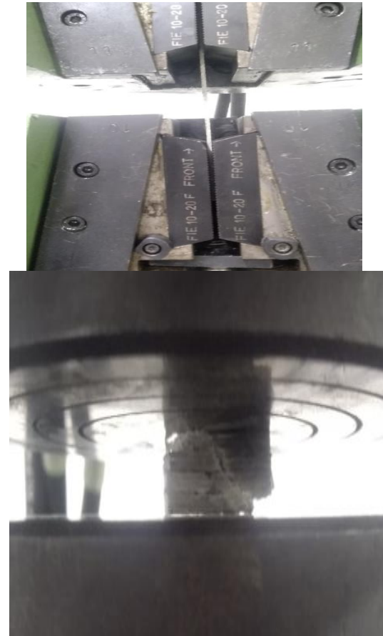
Figure 6: Specimens under UTS, flexural, Impact, and compression test
