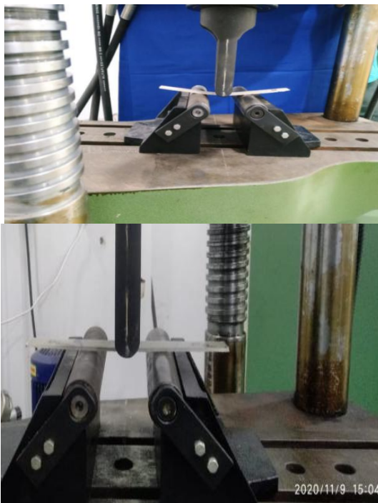
Figure 5: Specimens under flexural strength test
