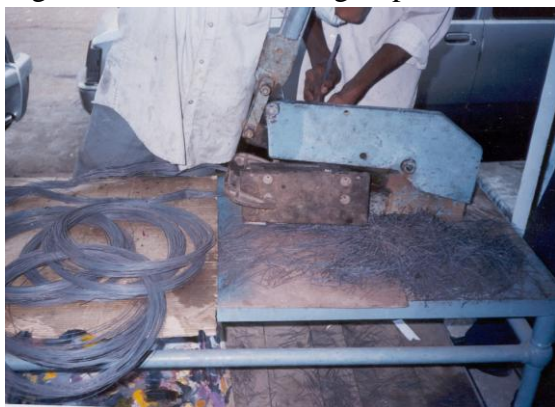
Fig 1.8.1 Chopping the steel fibre with shear cutting machine. Fibres like steel can be adopted towards
