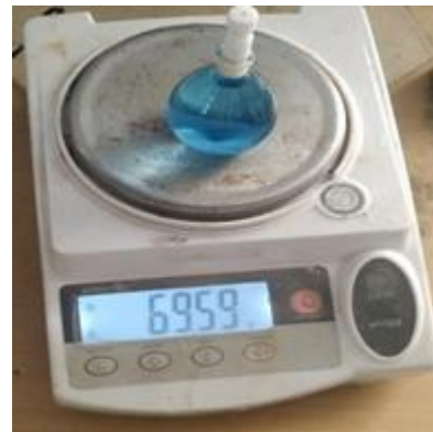
Fig. 2.4: Specific gravity of cement
